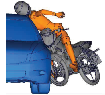
Figure 10. Still images from the videos of a full-scale motorcycle to moving car crash test. The left-hand column of images comes from the physical test and the right-hand column of images from the finite-element simulation.
