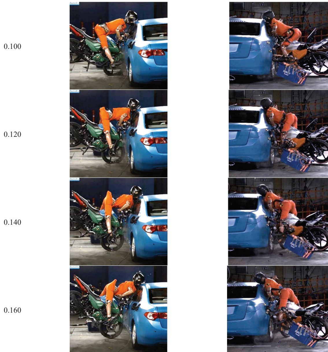
Figure 7. Still images from the video footage of two full-scale motorcycle to car crash tests. The left-hand column of images comes from the stationary car test and the right-hand column of images from the moving car test.
