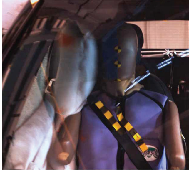
Figure 14. Still image of the WorldSID-50M from the 2019 Mini Cooper Convertible crash test (11614) showing ATD interaction with the combination head/torso airbag and intrusion which caused the arm, shoulder rib, and thorax ribs to experience similar loading.
