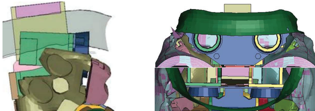
Figure 30. Illustration of the possible interaction between the belt (green) and the abdomen internal plate (blue) in a simulation of the standard abdomen with the FE model. The IR-TRACCs are materialized by the line at the center of the backing plate flared overload cones and the abdomen and jacket are not shown. For a belt pull, the belt motion and IR-TRACC compression can be limited by the internal plate (laterally) and the flared overload cones (anteriorly).
