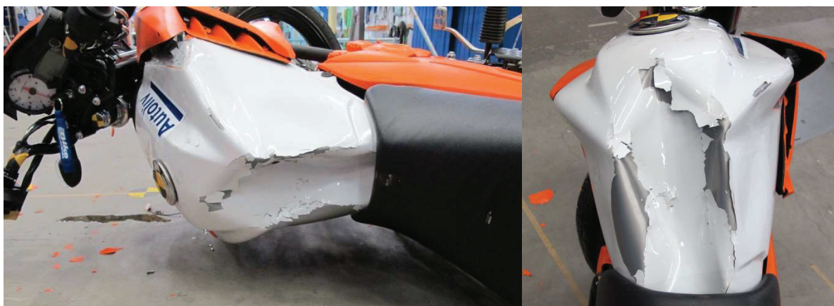
Figure 8. Images after the moving car test, showing the deformation of the fuel tank caused by the rider's pelvis.
