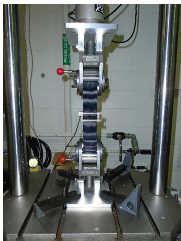
Figure 2. Harness webbing tensile test setup (left) and force time-history of Instron ® uniaxial tensile tester load cell and supplemental belt gauge (right).
