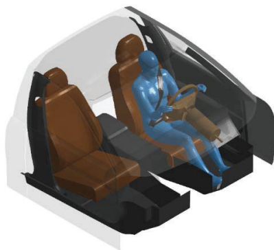
Figure 1. Far-side impact simulation setup with F05-OS+B model settled in a far-side simplified vehicle model
