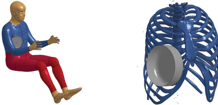
Figure 4. Validation of ribcage subsystem response by means of oblique pendulum impact tests according to Viano (1989)
