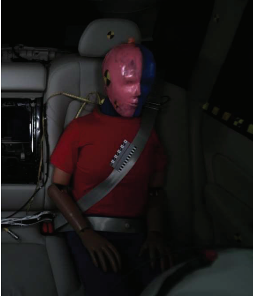
Figure 9a. CF19023 (XC60) Pre-impact belt position
