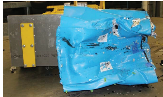
Kerb mass: 2480kg Deformation SD: 89mm Bottoming out: No
