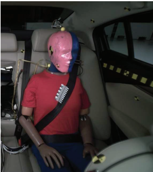
Figure 9c. CEF2109 (6) Pre-impact belt position
