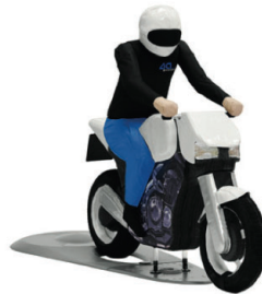
Figure 1. 4activeMC motorcycle target with the 4activeFB-small platform
