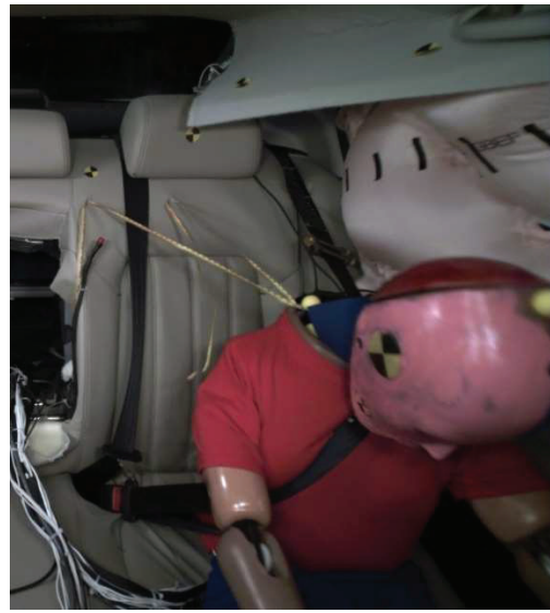
Figure 9d. CEF2109 (6) belt position @ maximum excursion
