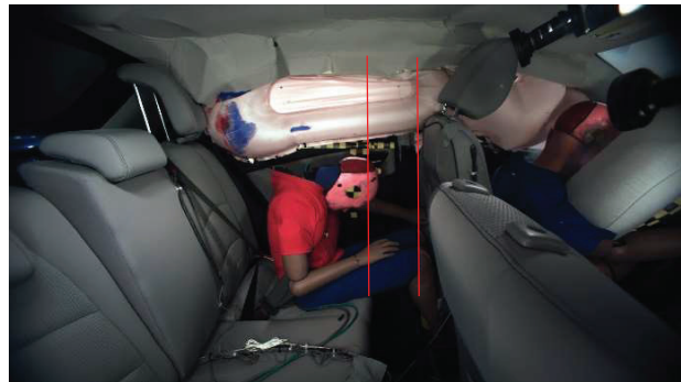
Figure 2b. Photo at 110 ms showing the front seatback moving in phase with the rear-seat occupant's excursion
