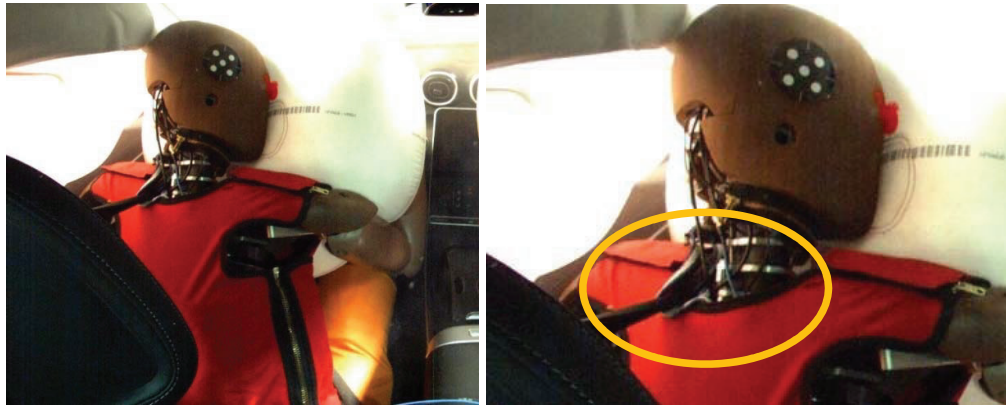
Figure 10: THOR diagonal belt slippage
