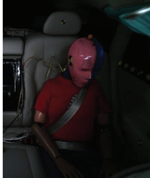
Figure 9b. CF19023 (XC60) belt position after pretensioning
