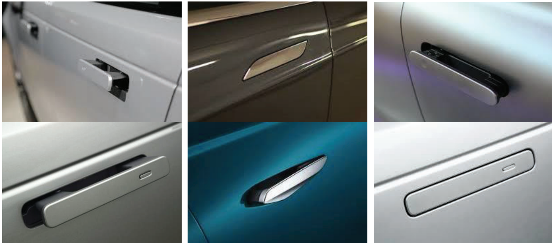
Figure 5. Example of recent door handle designs. Euro NCAP's assessment of post-crash safety includes a check that electric door handles still function post-impact.
