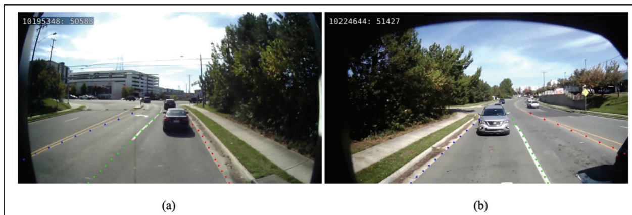
Figure 4. Video images. Example of lane detection using ultra-fast lane detection algorithms on the (a) front and (b) rear video from the ego vehicle’s camera.
