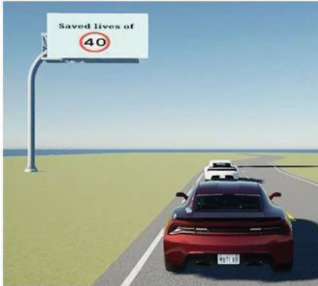
Figure 7. Detection of billboard by white EV with ISA functionality followed by a red POV.
