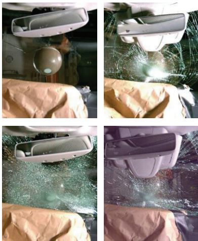
Figure 6. Windscreen behaviour during headform tests: no breakage (upper row, left), typical pattern (upper row, right) and atypical windscreen fracture modes (lower row) (source: BAST)
