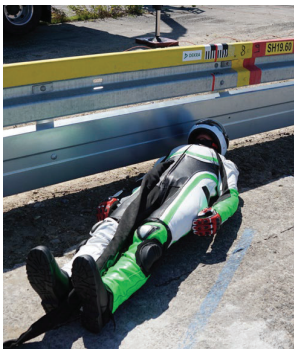
Figure 3: Impact according CEN/TS 1317-8:2012 (source: BAST)
