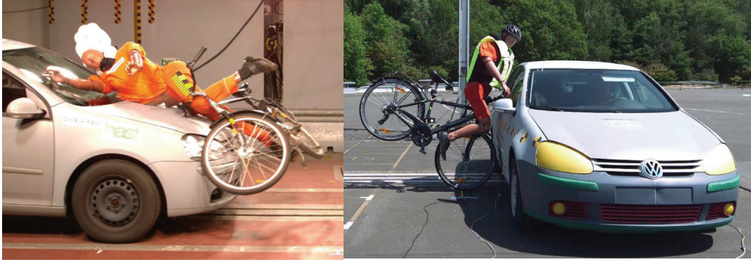
Figure 7 + 8. Vehicle to bicyclist accident simulation with different airbag based personal protective equipment: head protection system (left, fig. 7) and airbag vest (right, fig.8) (source: BAST)
