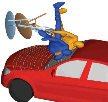
Figure 5. Vehicle corner to bicyclist impact simulation with bicycle speed of 15km/h (orange) and 25km/h (blue) (source: BAST)
