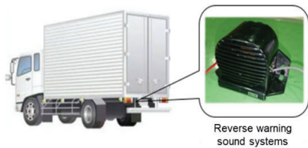
Figure 3. Installation example of reverse warning sound systems
