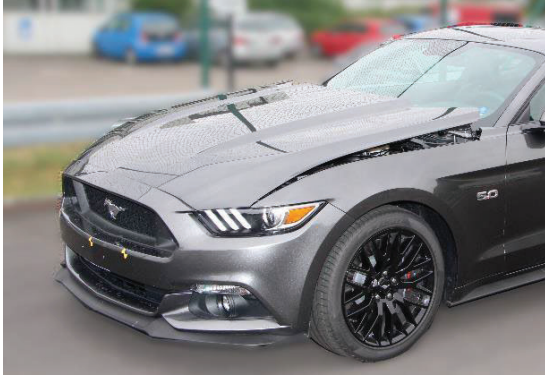
Figure 9. Vehicle with pop up bonnet as deployable pedestrian protection system (source: BASt)
