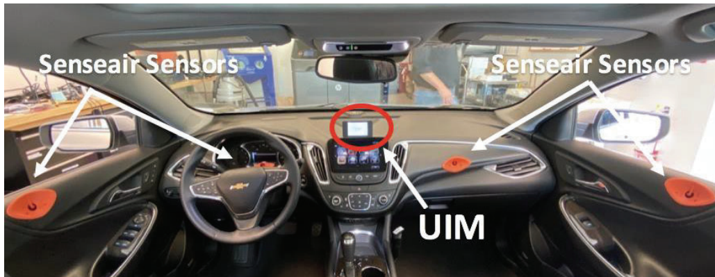
Figure 13. Position of the breath sensors and user interface module on the driver (left) and passenger sides of the vehicle.
