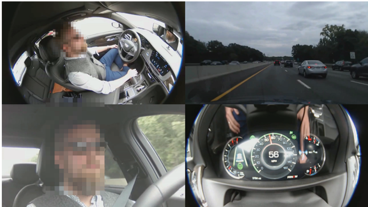
Figure 1. Example of hands-free, legs-free driving in the Cadillac CT6 with SC engaged as captured by the four RIDER cameras, including: the driver's face, in cabin view, instrument cluster, and the view of the forward roadway.
