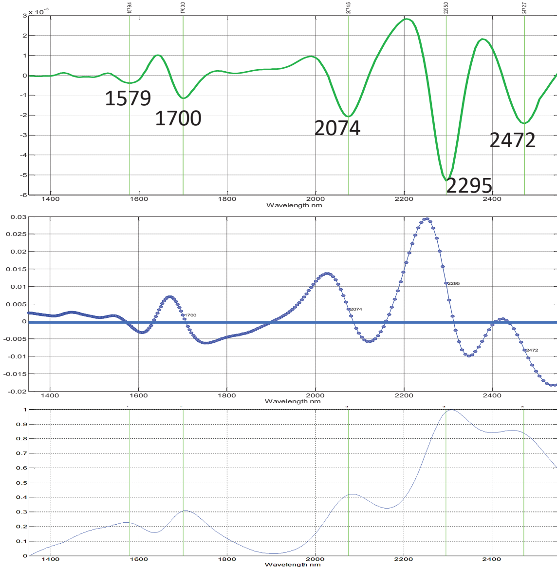
Figure 2. Shows the alcohol NIR spectrum, (Bottom) First Derivative (middle) and Second Derivative (Top) of from NIR-AS (unit #212) spectrometer.
