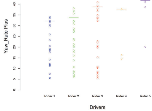
Figure 2: Values of the yaw rate at known accident locations with the 90% quantiles (signified by horizontal bars in the graph) of each rider being represented by a horizontal bar in the data. Panel a) depicts values of the yaw-rate minus at left curve accidents, while Panel b) depicts values of the yaw-rate plus at right curve accidents. Data while following other vehicles or having poor satellite connection has been removed.
