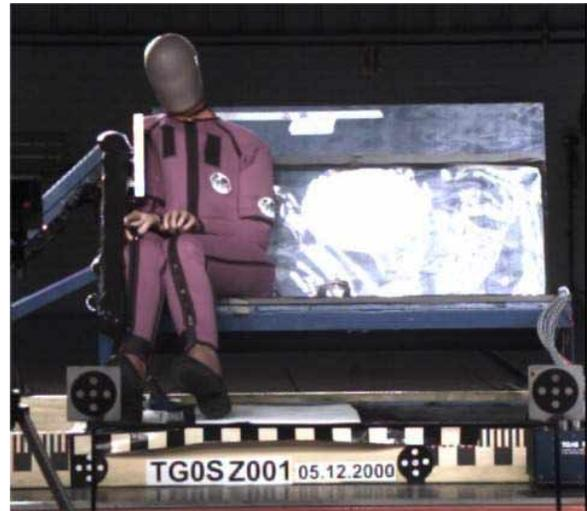
**FIGURE 11 Dummy impacting load wall in sled test**
