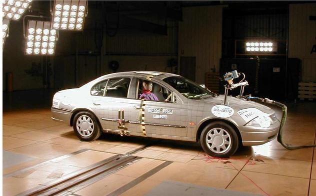
**FIGURE 12 Dummy in Falcon prior to impact**
