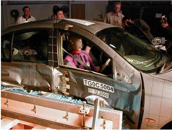
**FIGURE 9 Falcon after MDB test**
