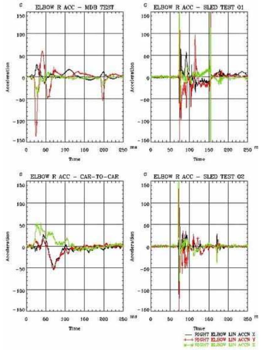
FIGURE B 26 Right elbow accelerations (CFC 1000)
