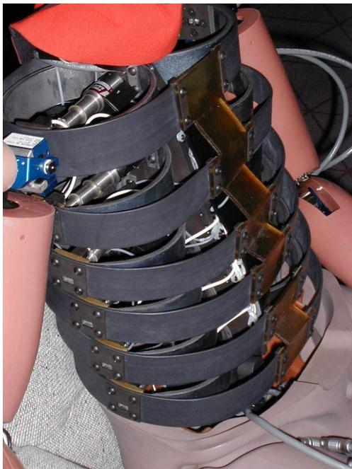
**FIGURE 3 View of the WorldSID prototype shoulder, thorax and abdomen ribs**
