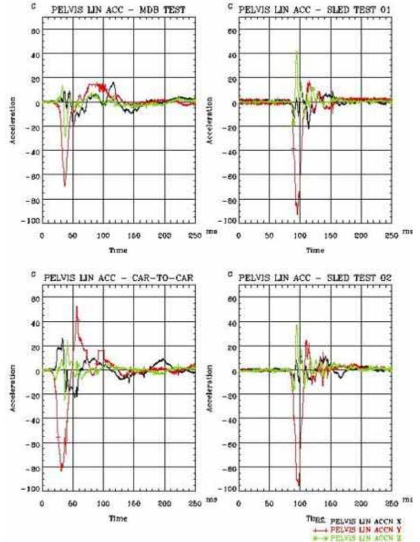
FIGURE B 14 Pelvis linear accelerations (CFC 1000)
