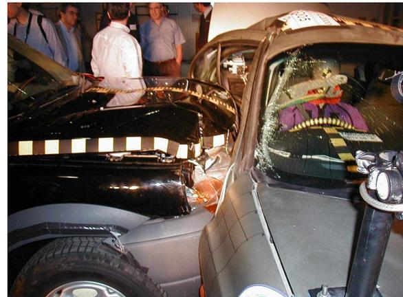
**FIGURE 14 Falcon and Freelander post test.**
