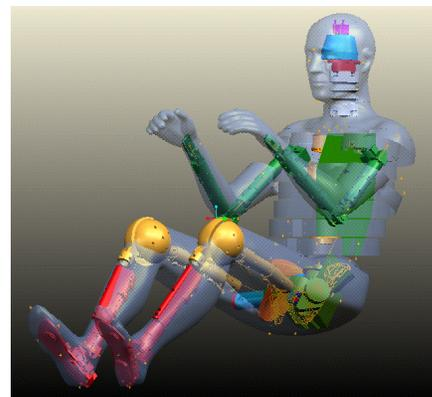
**FIGURE 1** CAD image of the WorldSID prototype dummy
