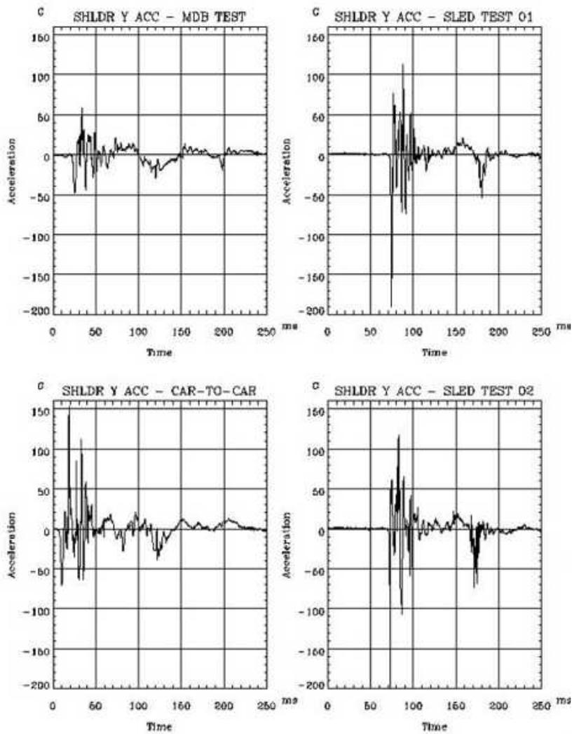
FIGURE B 23 Shoulder y-axis linear accelerations (CFC 1000)
