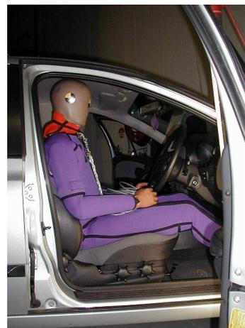
**FIGURE 8 WorldSID dummy seated in Falcon prior to final positioning.**
