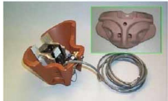
**FIGURE 4 Pelvic structure and pelvis flesh (insert).**
