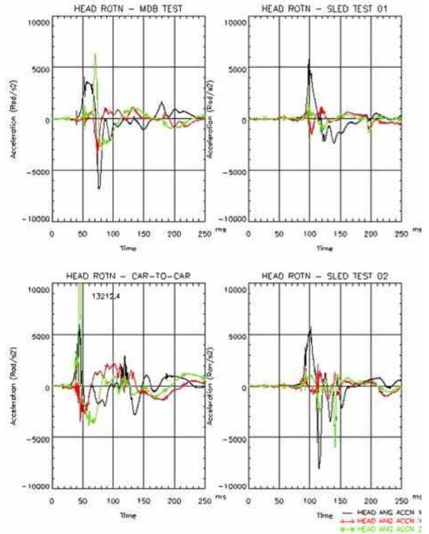
FIGURE B 2 Head angular accelerations (CFC 1000)
