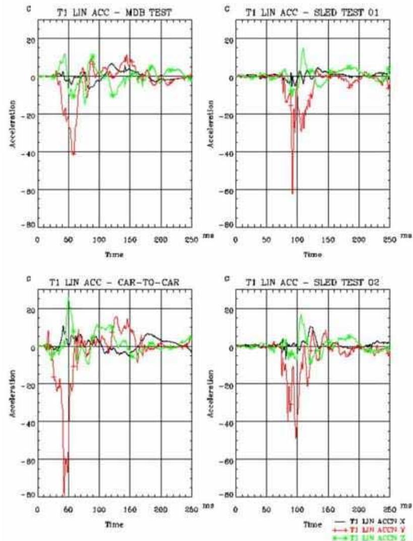
FIGURE B 8 T1 linear accelerations (CFC 180)
