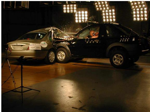
**FIGURE 13 Falcon with WorldSID impacted by the Freelander.**
