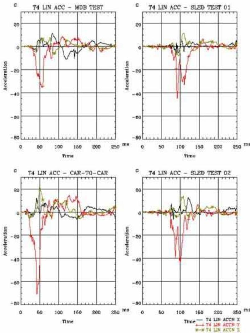
FIGURE B 9 T4 linear accelerations (CFC 180)
