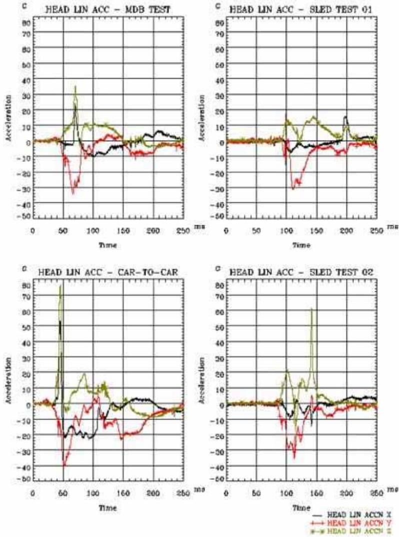
FIGURE B 1 Head linear accelerations (CFC 1000)
