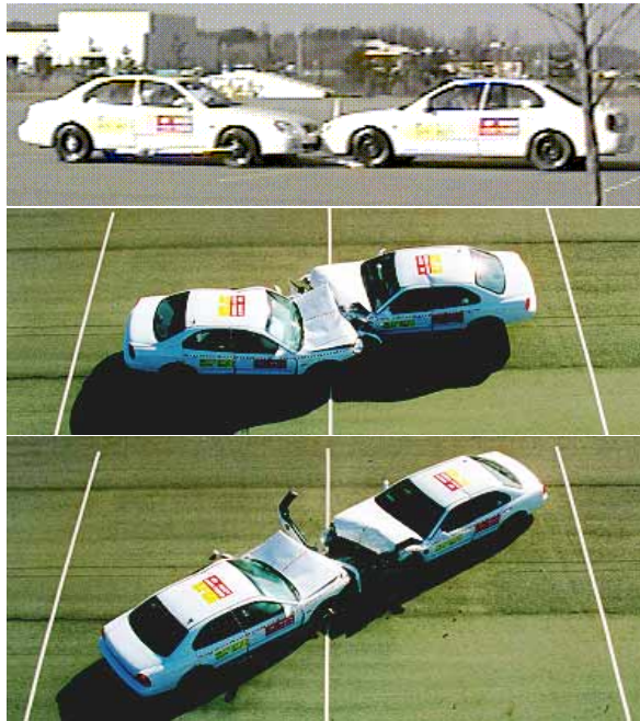
Figure 3. Car-to-car 50% overlap offset crash test. (midsize vs. midsize, 50km/h each)
