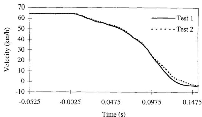
**Figure 1. 1995 Ford Taurus Vehicle Longitudinal Velocity.**
