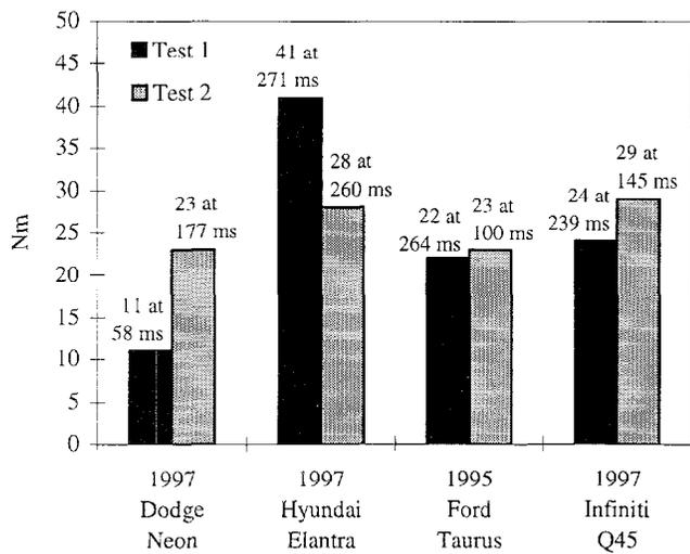
Figure 14. Comparison of Neck Extension Bending Moment.
