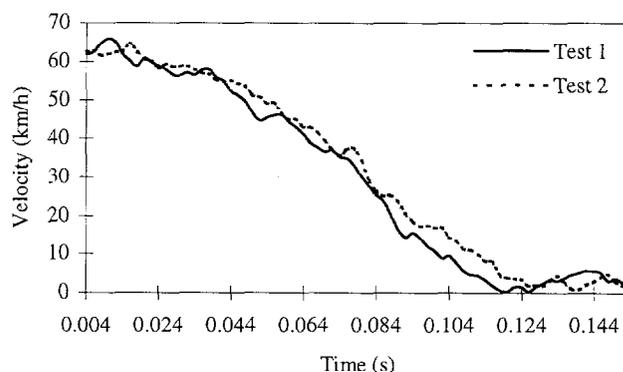
**Figure 3. 1997 Hyundai Elantra Vehicle Longitudinal Velocity.**
