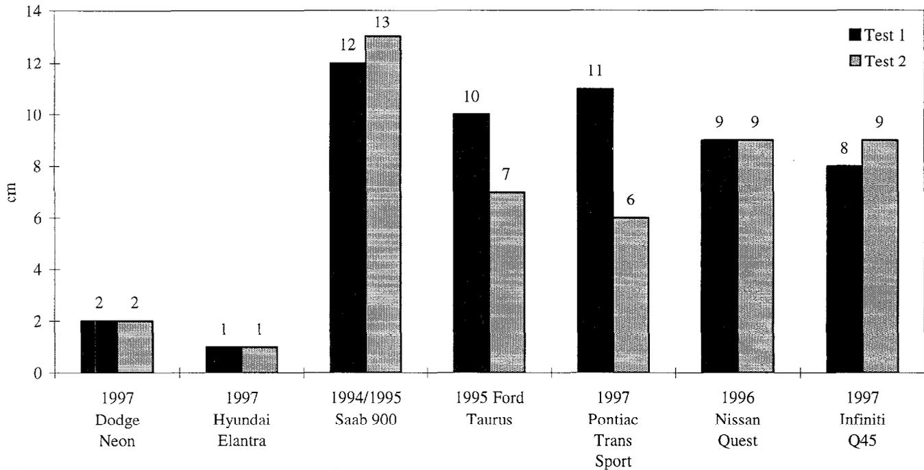
Figure 11. Comparison of Vertical Steering Column Intrusion.
