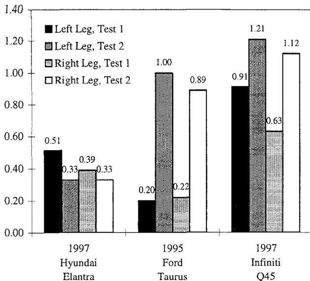
Figure 21. Comparison of Lower Tibia Index.
