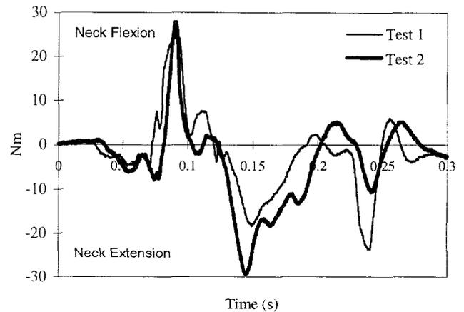
Figure 15. Neck Bending Moment - Infiniti Q45 Tests
