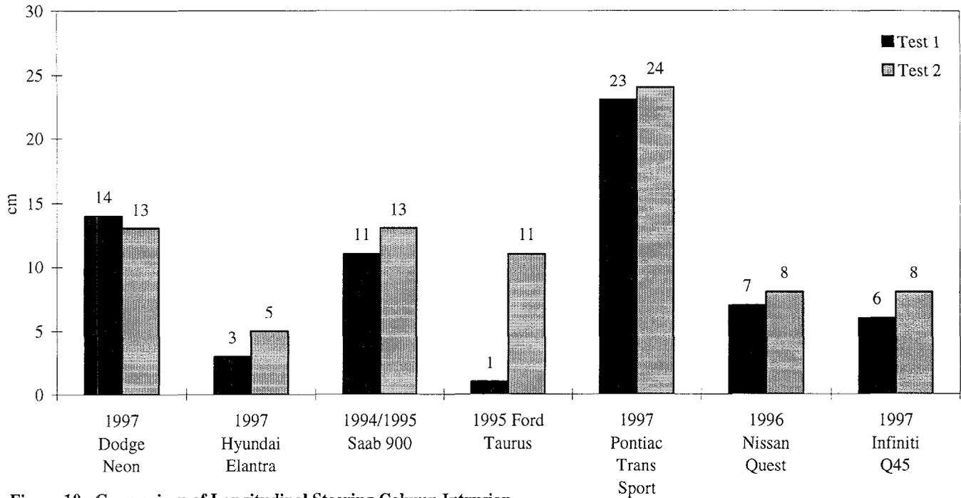
Figure 10. Comparison of Longitudinal Steering Column Intrusion.
