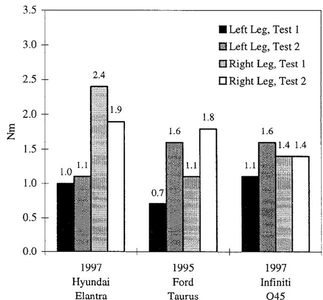
Figure 20. Comparison of Lower Tibia Axial Forces.
