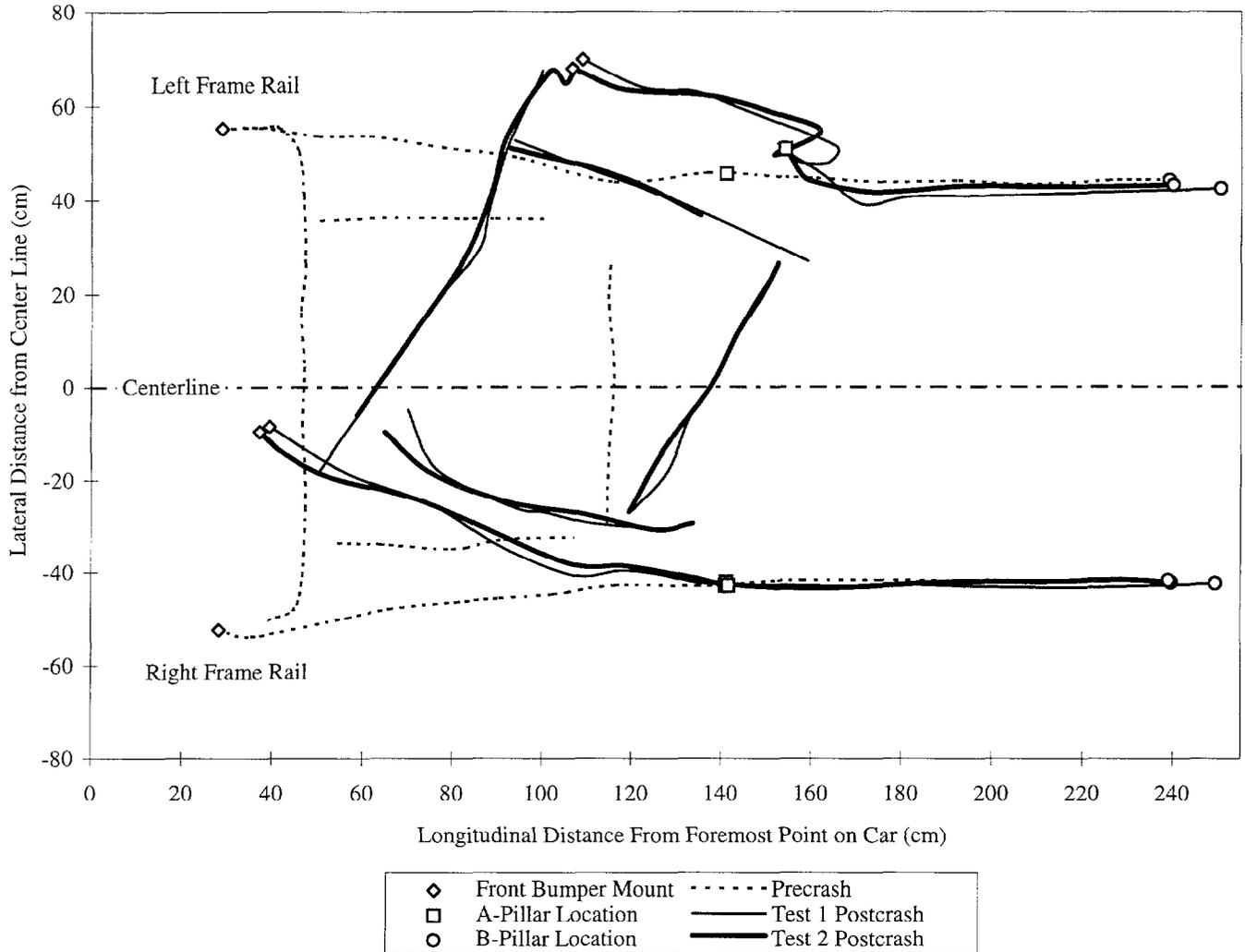
Figure 8. 1997 Pontiac Trans Sport Frame Rail Deformations, View from Below.
