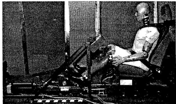
Figure 3. Foot well intrusion system mounted on a platform
