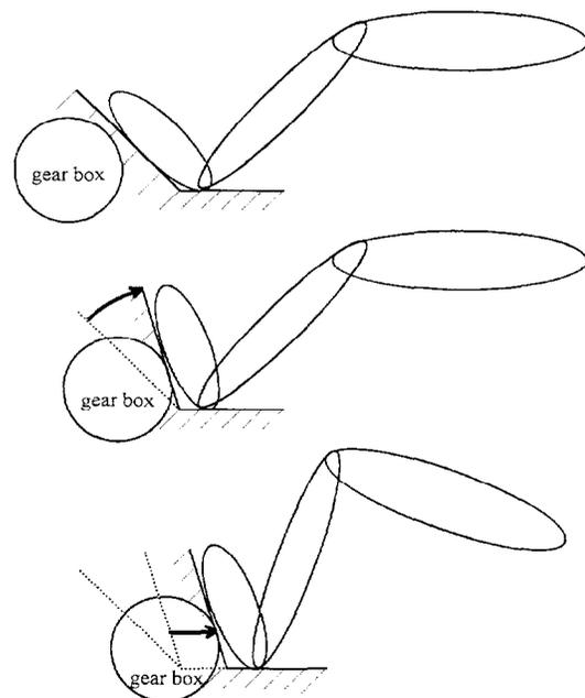
**Figure 1. Principle of foot well intrusion during crash.**
