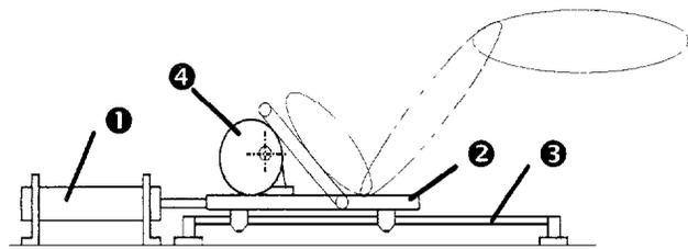
Figure 2. Principle assembly of the foot well intrusion system.
