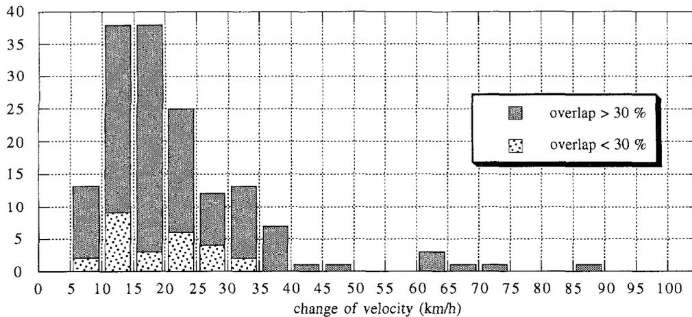
Figure 1. Number of impacts with an overlap more and less than 30% at different  $\Delta V$ 's.
