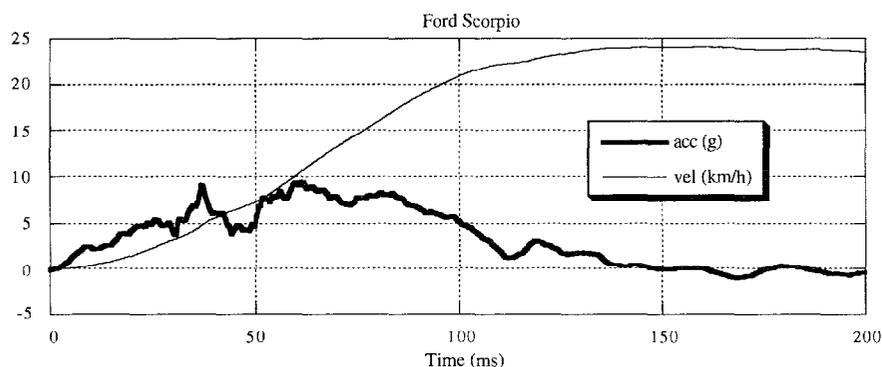
Figure 8. Crash pulse and change of velocity for the Ford Scorpio.
