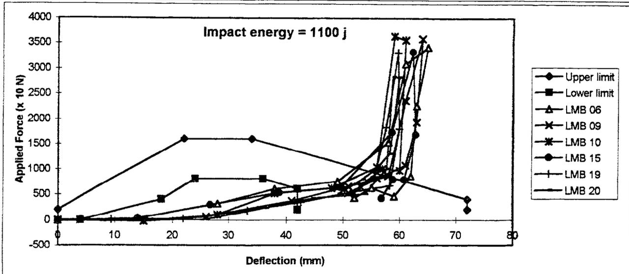
Figure 17 : EUROSID-1 Pelvic impact tests
