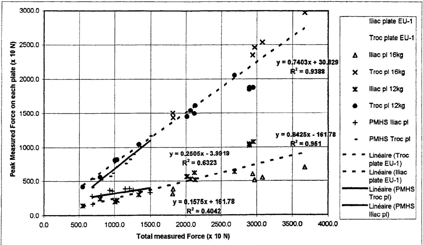
Figure 11 : Measured force on pubic symphysis and total applied force on EUROSID-1 pelvis
