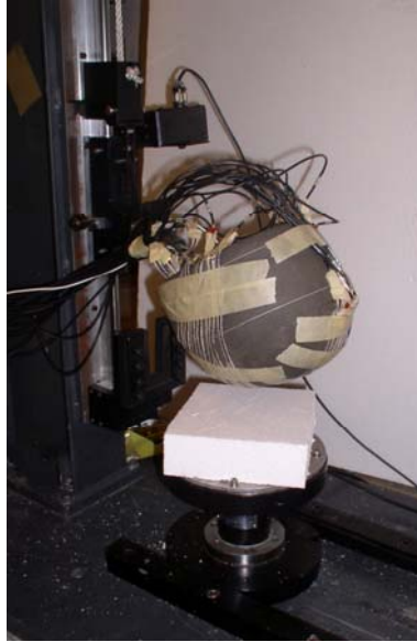
Figure 6: Test setup of instrumented headform impacting EPS.
