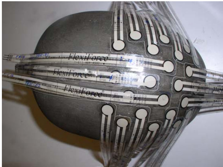
Figure 5: Thin film sensors attached to DOT size medium headform.
