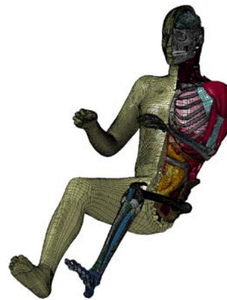
Figure 8. Oblique view of the M50 model, seated, with half the flesh layer elements not visible, to show underlying structures.
