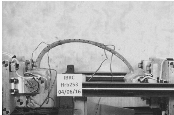
Figure 2: Exemplar human rib in the test fixture prior to testing
