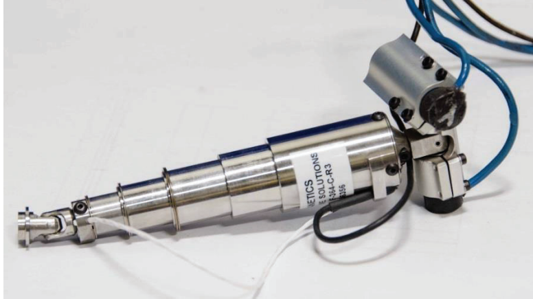
Figure 5: IR-TRACC installed in double gimbal assembly
