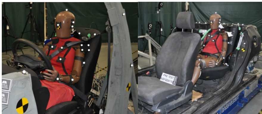
Figure 2. THOR-05F positioned in the front seat (left) and rear seat (right) sled bucks.
