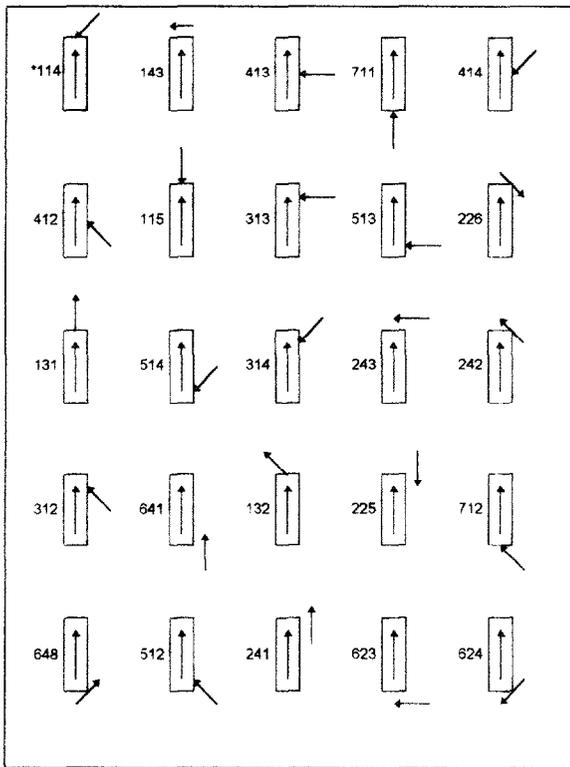
**Figure 16 Motorcyle/car impact configurations defined in ISO/DIS 13232**
