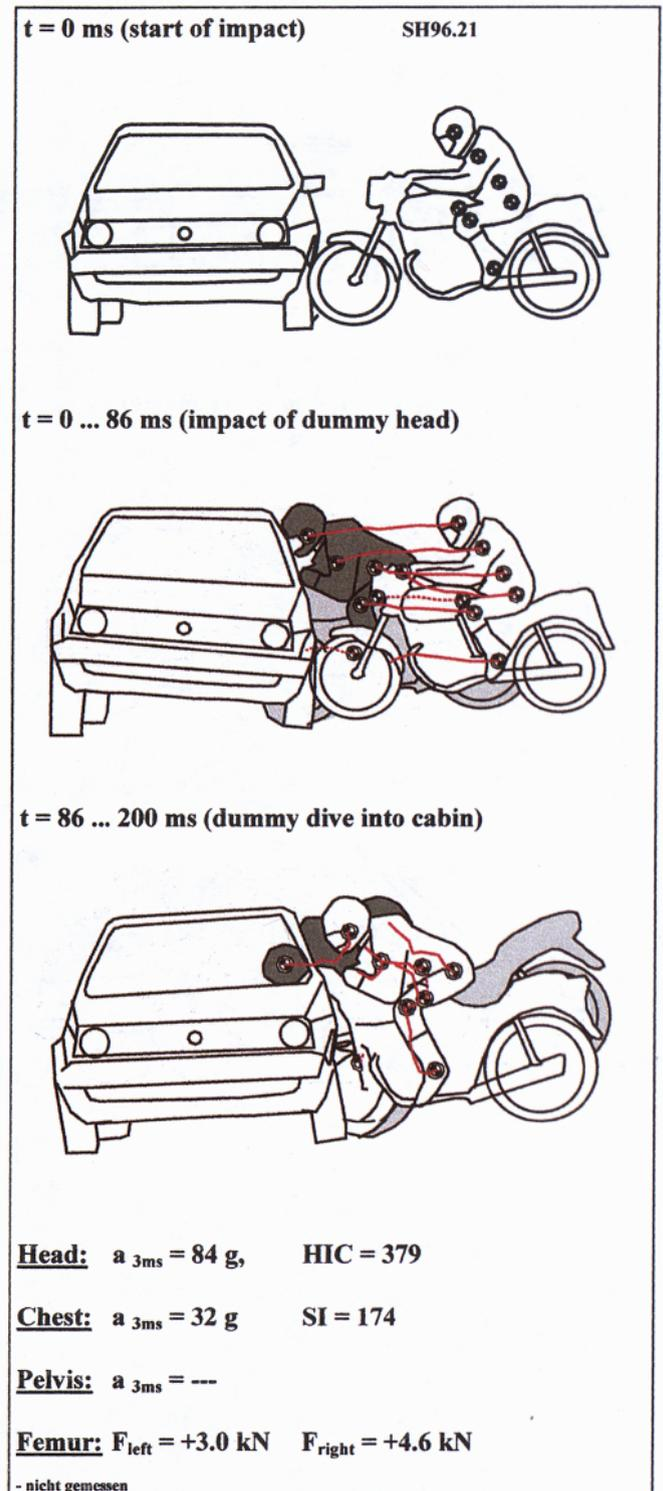
Figure 23. Results of film evaluations of a full-scale crash test between moving motorcycle and stationary passenger car and measured head, chest and femur loadings of the dummy (Configuration 413 in ISO/DIS 13232)
