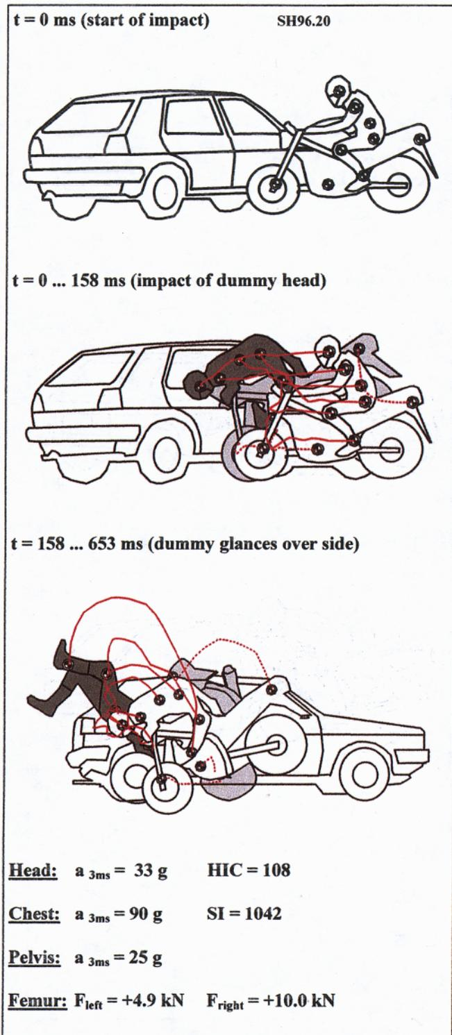
Figure 22. Results of film evaluation of a full-scale crash test between moving motorcycle and moving passenger car and measured loadings of the dummy (Configuration 414 in ISO/DIS 13232)
