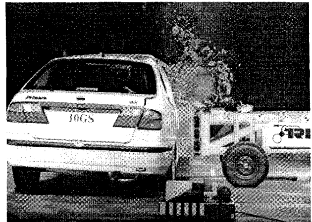
Figure 2. Euro NCAP Mobile Deformable Barrier Side Impact Test at 50 km/h
