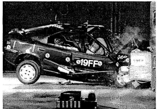
Figure 7. Loss of Passenger Compartment Integrity due to Overloading.
