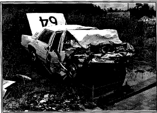
Figure 8. High speed frontal crash in which the driver was saved by the air bag.
