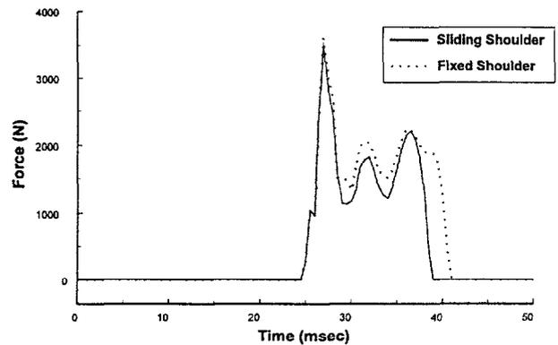
*Figure 6. ATB Simulation of Fixed vs. Sliding Shoulder.*
