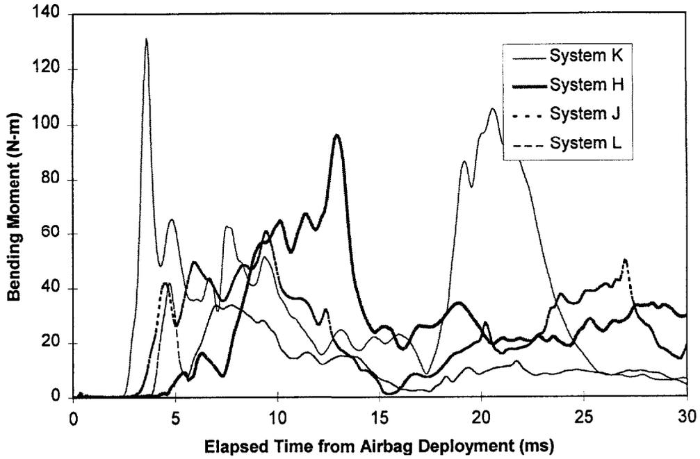
Figure 11. SAE Arm Midshaft Forearm Resultant Bending Moment (All Signals Filtered to SAE CFC-600).
