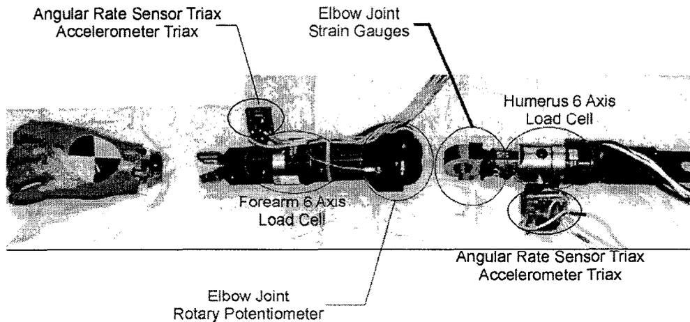
**Figure 1.** Picture of the SAE 5th Percentile Female Instrumented Arm (SAE Arm).
