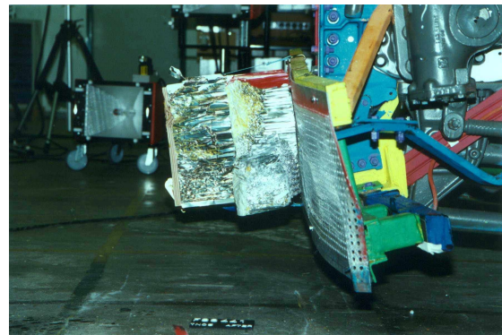
Figure 1. FUPD support and front elements of the truck deformed after a crash test carried out by TNO.
