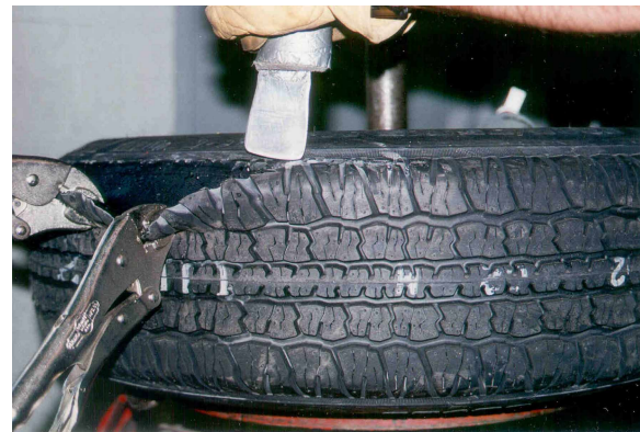
Figure 3. Tire Prep for Tread Separation Simulation.
