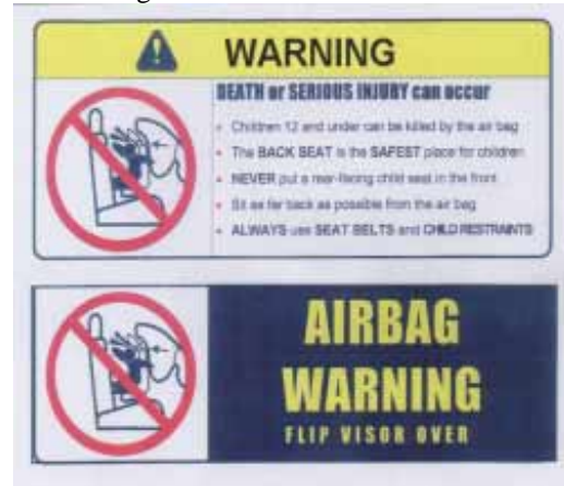
Figure 10. Example of airbag warning labels on sun visor in down and up position meeting both US and Euro NCAP requirements
