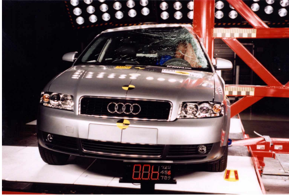
Figure 4. Euro NCAP side pole test
