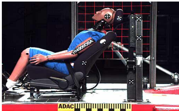
Figure 12. Rear impact whiplash protection test
