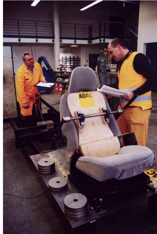
Figure 13. Seat stability test
