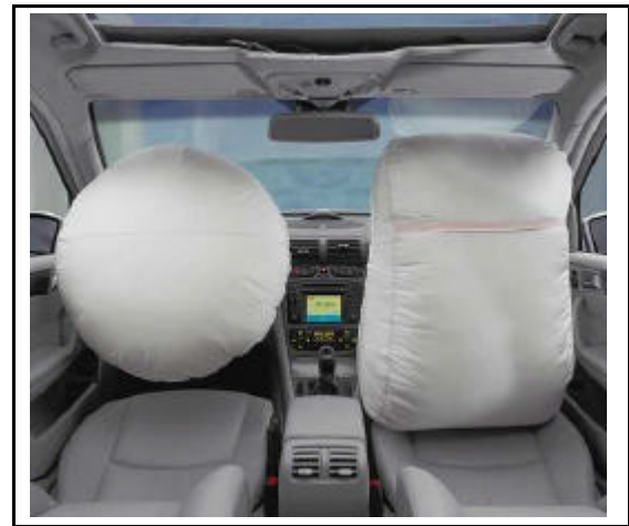
Fig. 3. Accident Severity Dependent Restraining Action of Driver and Front Passenger Airbag in the Mercedes-Benz C-Class
