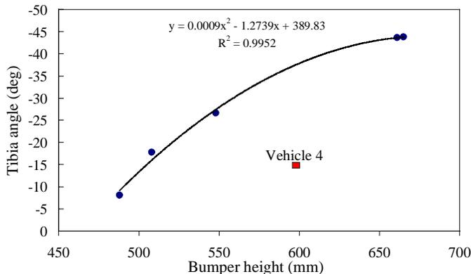
**Figure 16** Bumper Height and Tibia Angle
