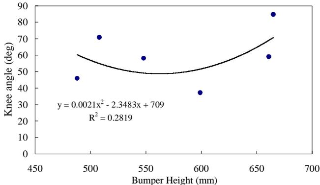
**Figure 14** Bumper Height and Knee Bending Angle
