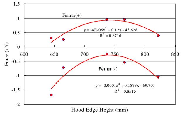
**Figure 12** Hood Edge Height and Femur Shearing Force
