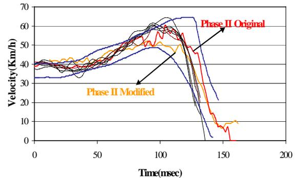
Figure 3 Resultant Head Velocity at 40 km/h
