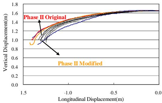
**Figure 5** Head Trajectory at 40 km/h
