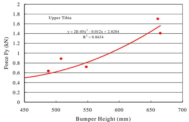
**Figure 13** Bumper Height and Upper Tibia Shearing Force
