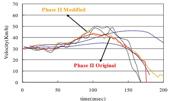
Figure 4 Resultant Head Velocity at 32 km/h
