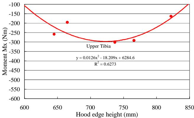
**Figure 10** Hood Edge Height and Upper Tibia Bending Moment
