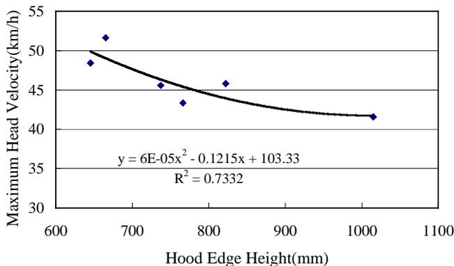
Figure 9 Hood Edge Height and Maximum Head Velocity
