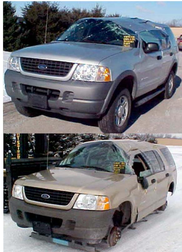
**Figure 1. The NHTSA test vehicles: at 5° pitch and 25° roll at top and at 10° pitch and 45° roll at bottom. The damage is similar only in that the damaged roof's contour follows the shape and angle of the platen used in the test.**
