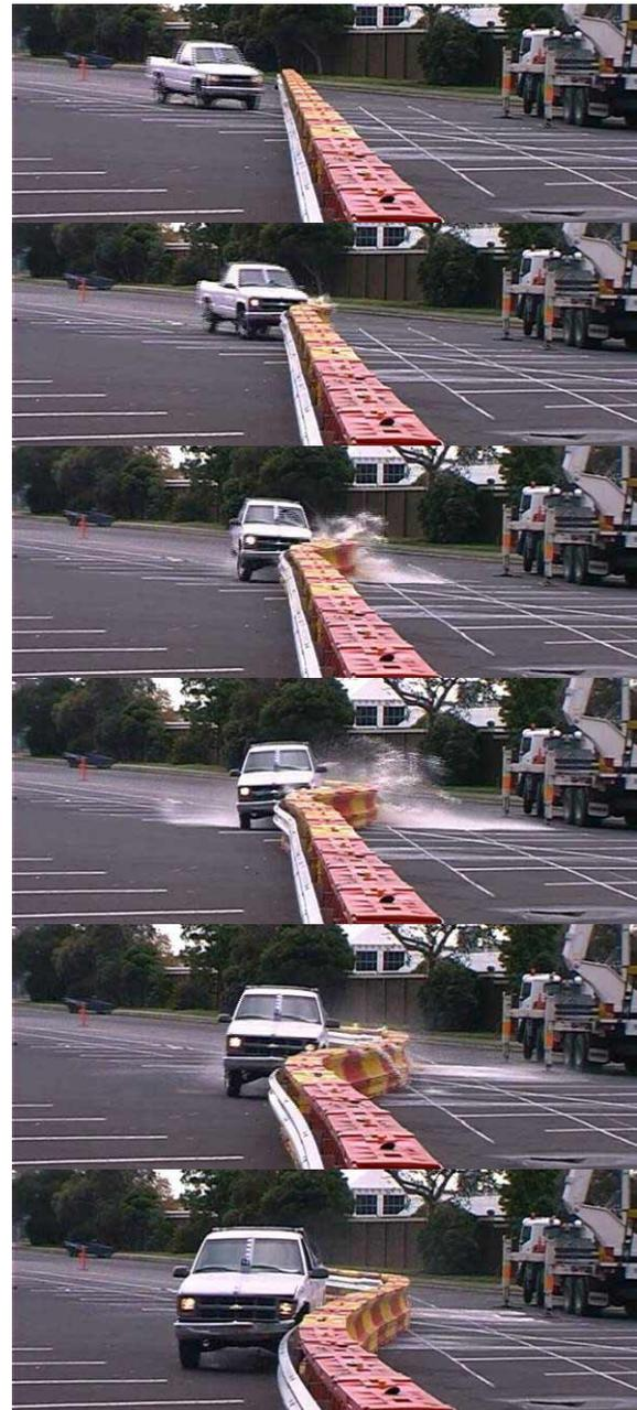
**Figure 20 Crash test of 2000 kg US pickup truck impacting barrier at 70 km/hr at 25°.**
