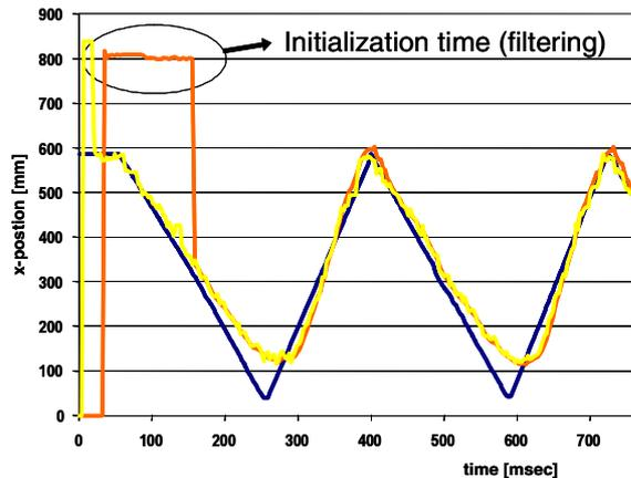
**Figure 15: Head tracker performance. Motion of test device (blue); Head position seen by the camera (yellow) vs position of head defined by tracker (orange)**
