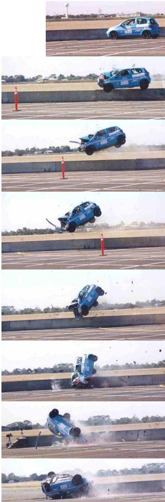
**Figure 7 Impact of Echo into New Jersey barrier at 80 km/hr and 45°.**
