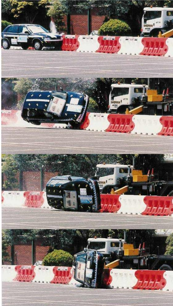
**Figure 16 Small car impact into plastic delineator barrier.**
