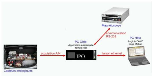
Figure 7. Instrumentation of MEGANE 1 (old vehicle)
