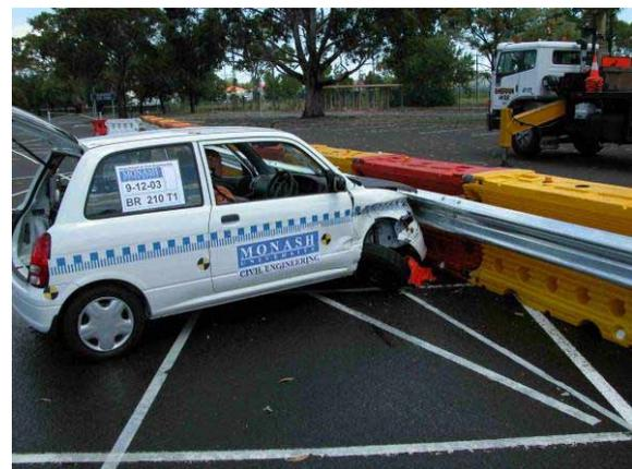
**Figure 17 NCHRP 350 Level 2 (70 km/hr at 20°) barrier crash test involving a Daihatsu car.**
