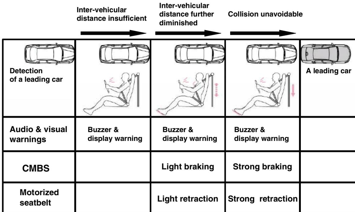
Figure 4. Operation modes of CMBS with motorized seatbelts.
