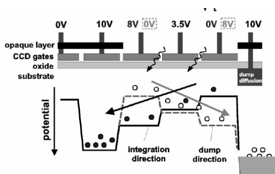
**Figure 4: Cross sectional view of the CCD pixel layout**
