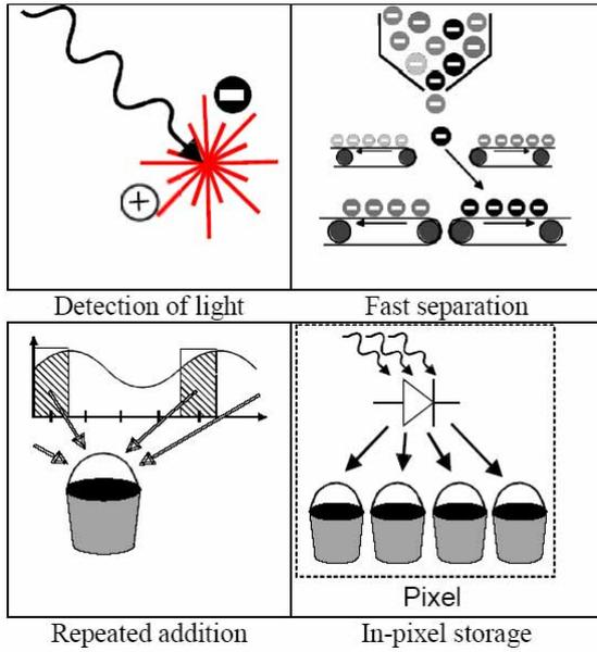
**Figure 5: Key function of the imager: Detection of light, fast separation of the generated electrons into the 4 different taps; repetition of the measurement until reliable signal generated and storage in of signal in pixel before reading out complete imager**
