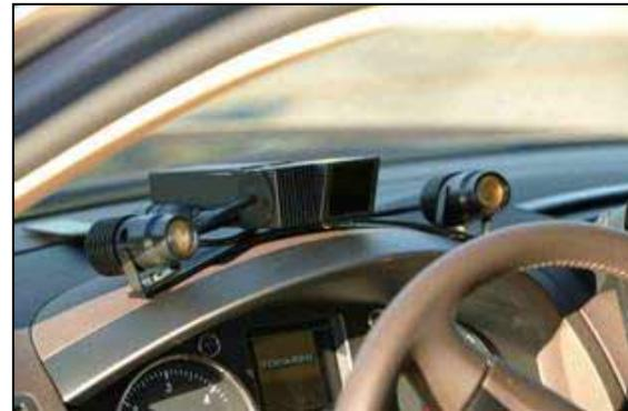
**Fig. 3:** Prototype of a video sensor in a VW car
