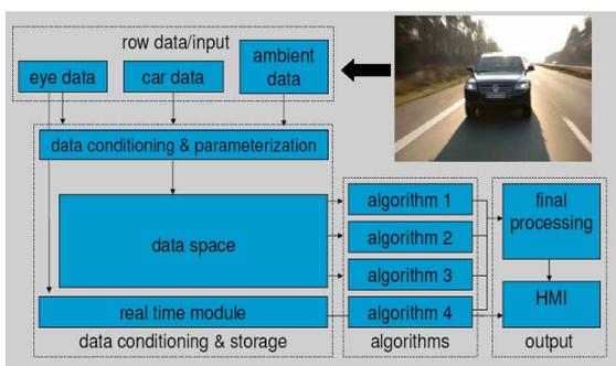
**Fig. 6:** Framework of driver's fatigue recognition algorithm
