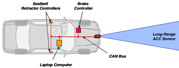
**Figure 4. Pre-crash prototype system configuration.**
