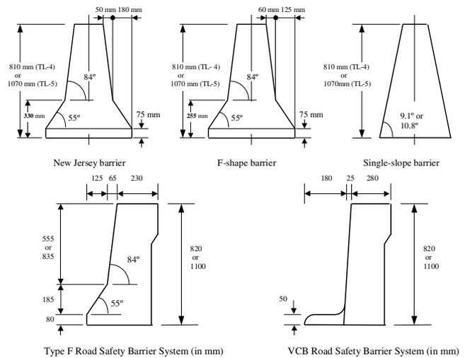
**Figure 1 Profiles of more common concrete barriers used in the USA and Australia**
