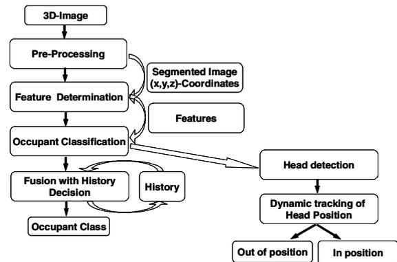
**Figure 6: Algorithm flowchart for static and dynamic classification**
