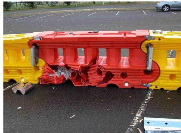
**Figure 18 Tears in barriers caused by engine rail spearing through plastic.**
