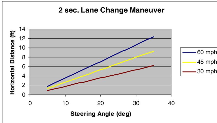
**Figure 2. Effect of Vehicle Speed on Horizontal Distance**
