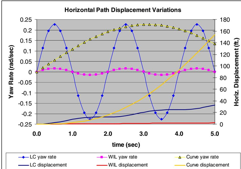
Figure 5. Summary Displacements vs. Yaw Rate Signals
