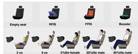
**Figure 10: Overview of different occupant types used for static classification**
