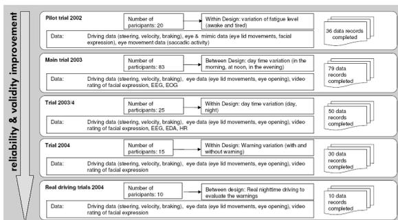
**Fig. 5:** Empirical basis of driver's fatigue recognition algorithm
