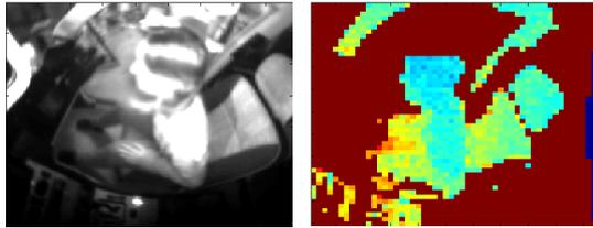
**Figure 7: (left side) intensity image of the scene. (right side) color coded distance raw image before preprocessing**
