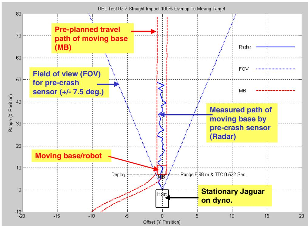
Figure 13. Test result rear-end scenario.
