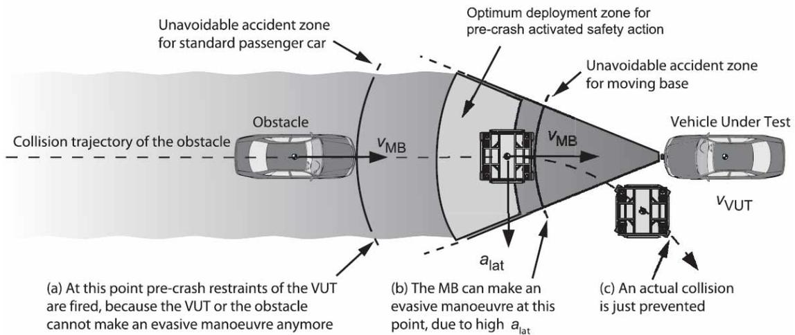
**Figure 9. Pre-crash test for a head-on collision scenario in VEHIL.**
