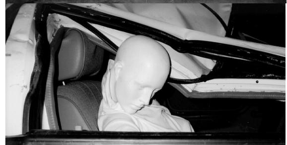
**Figure 15 Top: Damaged profile of vehicle from the Monash Series wire rope crash test. Middle and bottom: Similar crush profile and injury mechanism presented by Rechnitzer et al (1998).**
