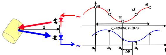
**Figure 3: Detected light intensity as a function of time. The sinusoidal modulation (top curve) of the illumination causes a periodically modulated signal in the receiver (lower area). The phase offset can be computed by evaluating the signal amplitudes  $a_0, \dots, a_3$  at 4 different temporal positions  $t_0, \dots, t_3$ .**
