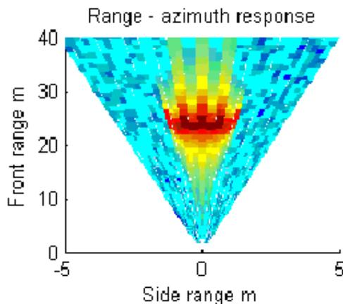
**Figure 17. Radar sensor model: view from sensor position and sensor output.**
