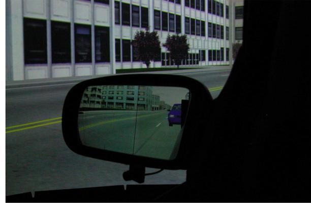
**Figure 8. View from driver's seat of convex mirror in NADS.**
