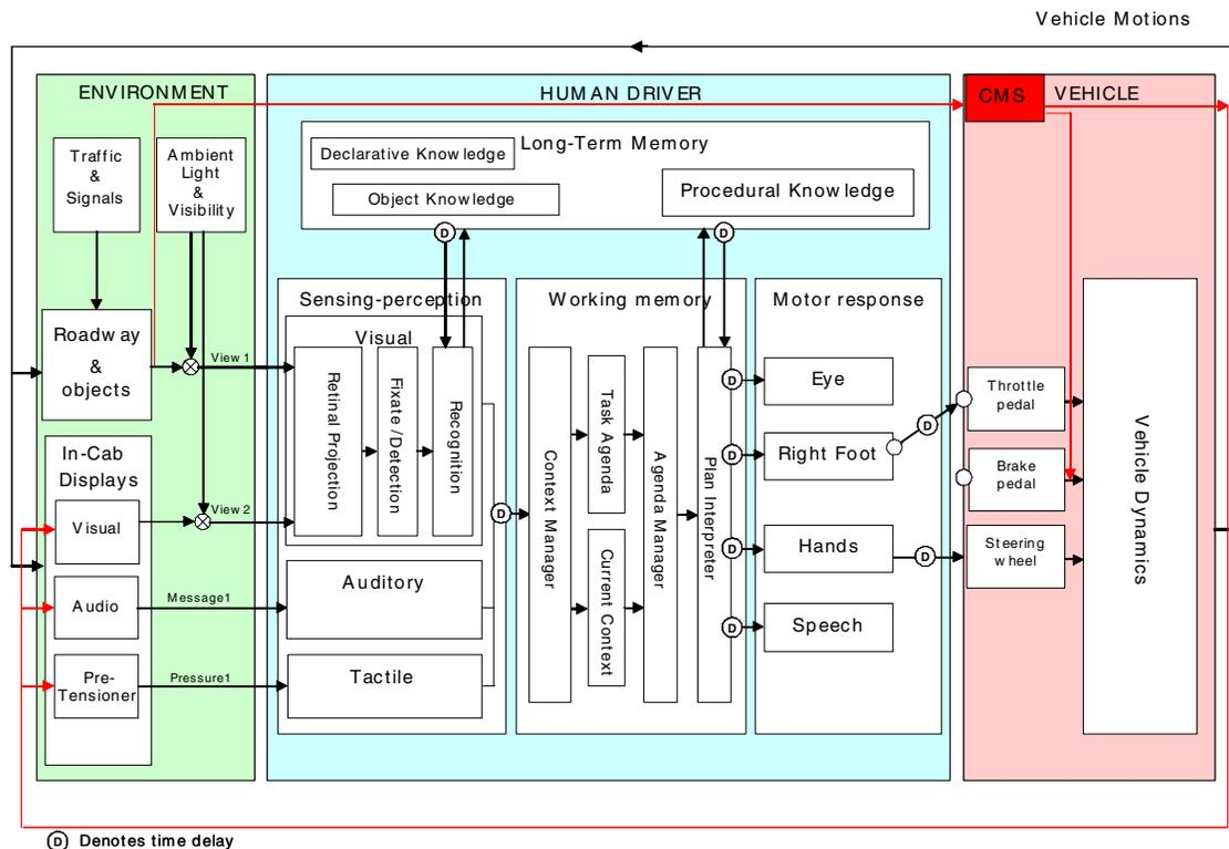
Figure 6. The concept of the simulation model
