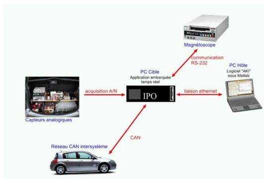
Figure 8. Instrumentation of MEGANE 2 (recent vehicle)
