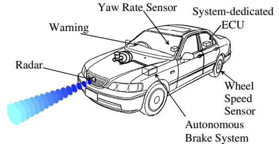
Figure 3. System configuration of CMBS.
