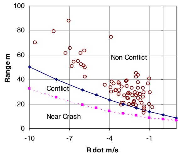
**Figure 7. Braking Response At Constant Speed Scenarios.**
