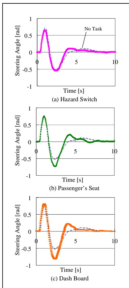
Figure 9. Steering Angle in Emergency Avoidance Compared with No Task.
