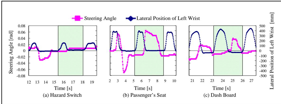
**Figure 6. Time History of Left Wrist Position and Steering Angle.**
