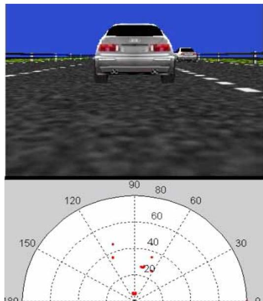
**Figure 16.** Laser scanner model: view from sensor position and sensor output.
