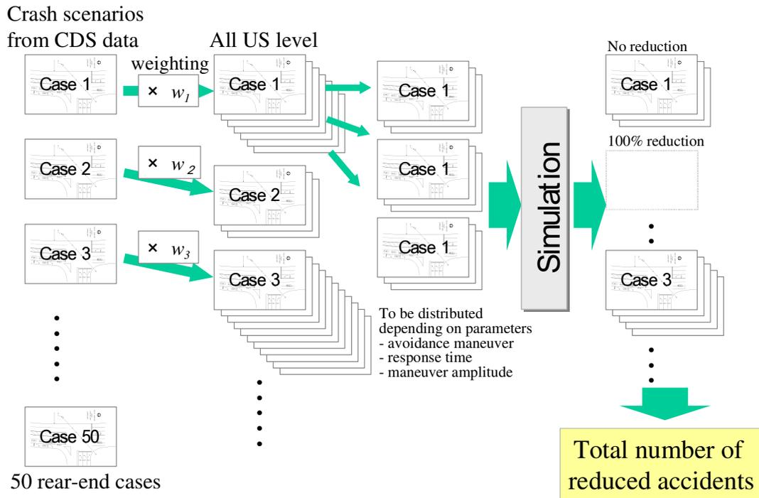
Figure 1. The concept of the effectiveness estimation method.
