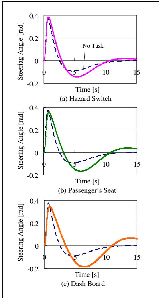
**Figure 10. Simulated Steering Angle in Emergency Avoidance Compared with No Task.**
