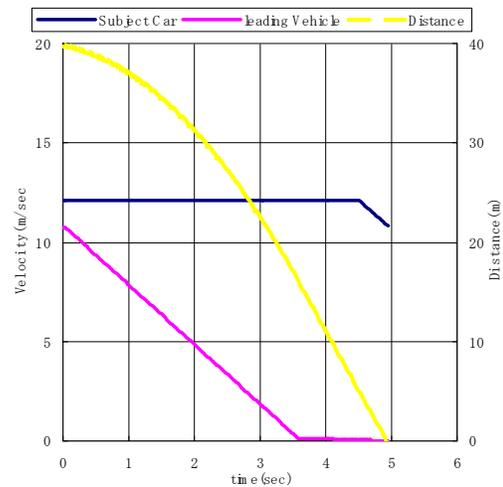
Figure 8. Simulation result of baseline condition without CMBS
