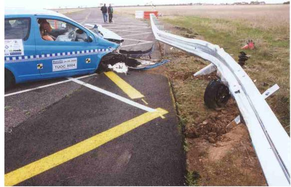
**Figure 12 Pocketing and under-ride into guardrail barrier – 80 km/hr at 45°.**
