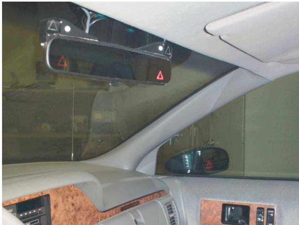
**Figure 1. TRW view from driver's seat of warning icons in and next to mirrors [2].**
