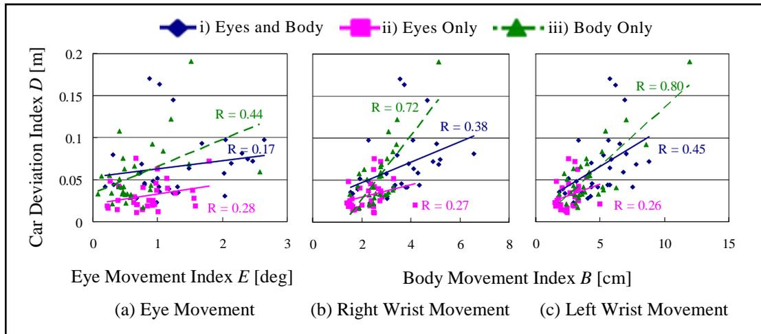
**Figure 5. Relationship between Car Deviation and Eye Movement, Body Movement.**
