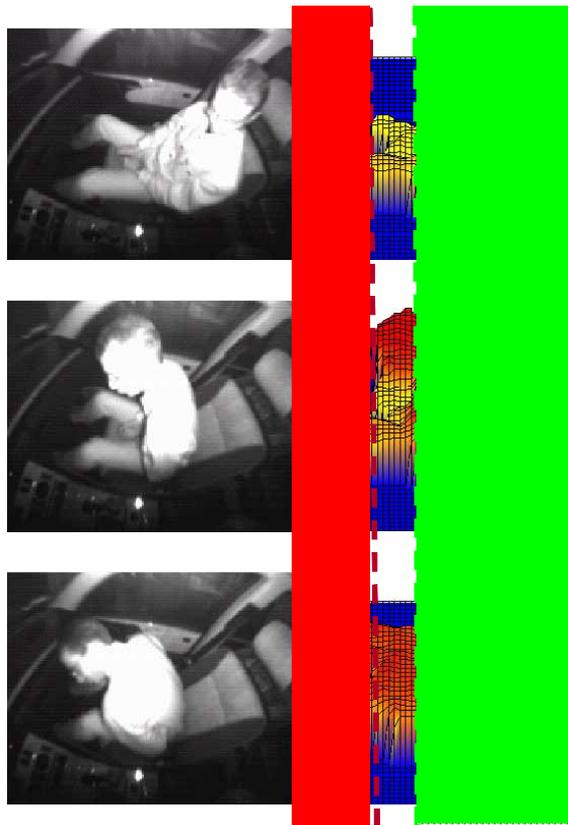
**Figure 9: Definition of occupant in position (top image), occupant out of position (middle image) and occupant in critical out of position (bottom image)**
