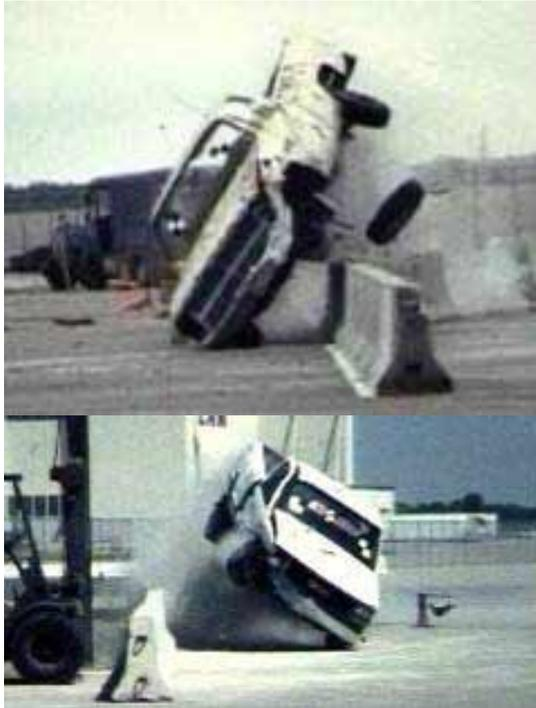
**Figure 10 Top: F shape moveable, Chevy C-20 at 99.4 km/hr and 26.4° Bottom: F shape fixed, Chevy ¾ ton at 99.8 km/hr @ 25.3° (after Sicking, 2004).**
