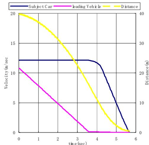
Figure 9. Simulation result with CMBS
