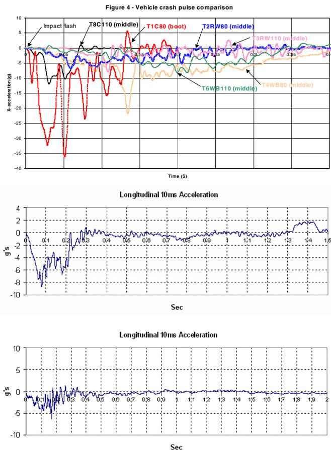
**Figure 19 Vehicle crash pulses from Monash test series: (top graph) where C=concrete (Figure 7), WB=W-Beam (Figure 12), W=wire rope (Figure 4 & Figure 15) and speed is 80 or 100 km/hr (see Grzebieta et al 2002 for details); and from water filled Level 2 barrier tests (middle graph is small car in Figure 17, bottom graph is pickup truck in Figure 20)**
