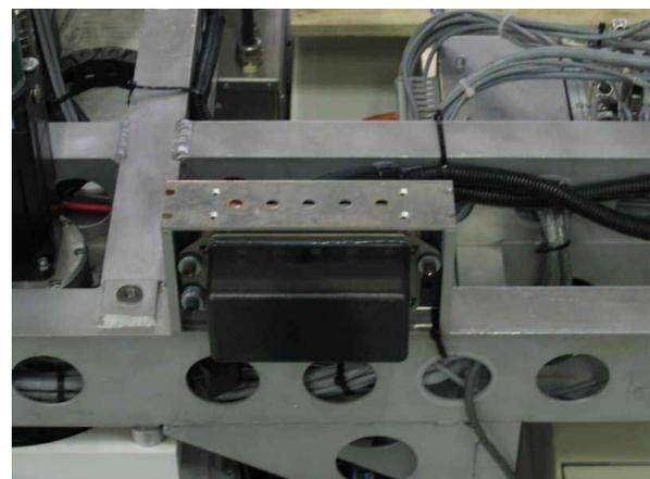
**Figure 11. Sensor mounted on the Moving Base.**
