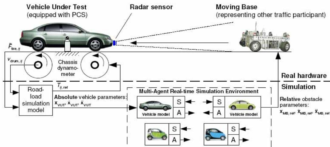
Figure 8. Working principle of VEHL [Gietelink, 2004].
