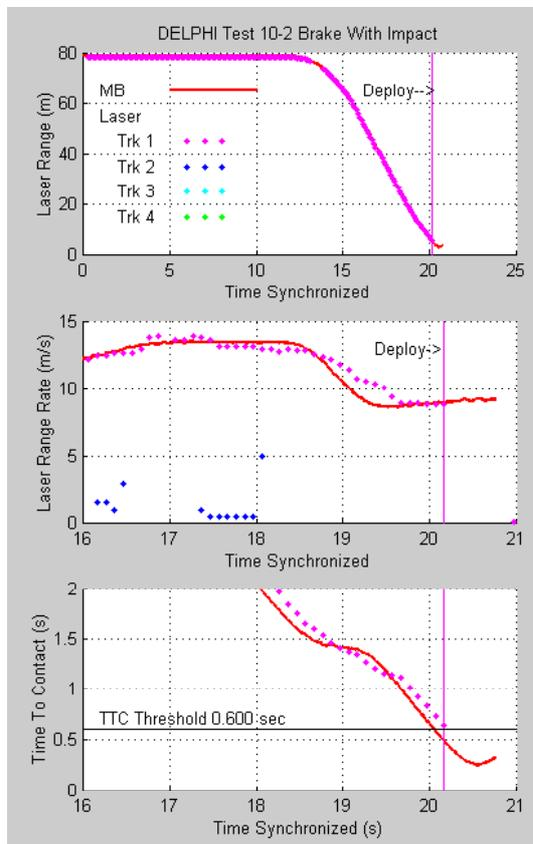
**Figure 15b.** Comparison of laser data to 'ground truth' data.
