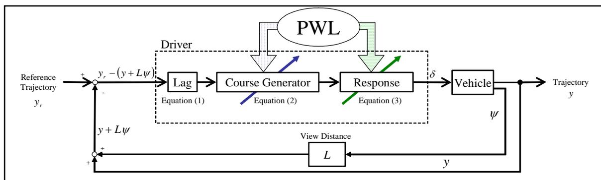
Figure 1. Driver Model with Physical Workloads.
