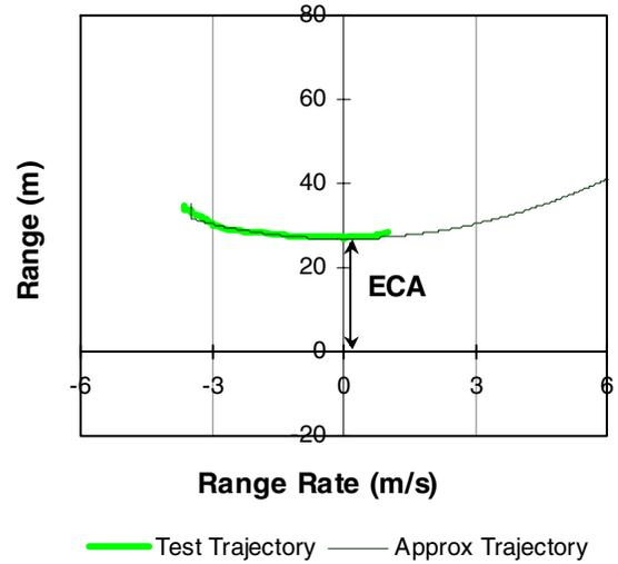
**Figure 4. Experimental And Approximate trajectories in Range/Range-rate coordinates.**
