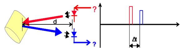
**Figure 2: Light pulse based time of flight. The turn around time of an emitted light pulse is measured and put into relation of the distance  $d=c \cdot \Delta t / 2$**
