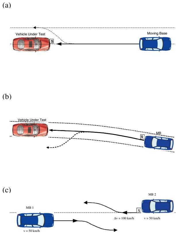
Relevant accident scenario (vehicle with pre-crash system indicated by thick orange arrows)
