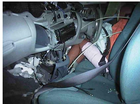
**Figure 8 External and internal crush deformation for 80 km/hr at 45° impact into concrete barrier.**
