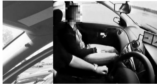
Figure 6. Showing the side camera location on the A-pillar and a sample of the camera output.
