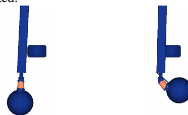
Figure 4. Simulation setup of Q3 dummy neck pendulum test just before impact (left) and at time of maximum neck bending (right)
