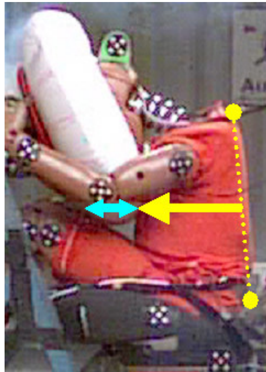
Figure 11. Double pretensioning reduces chest forward displacement
