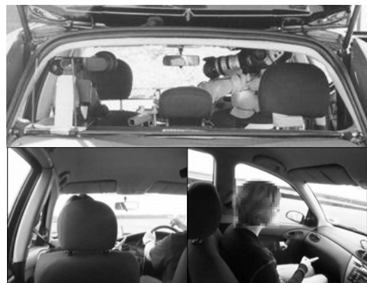
Figure 7. Showing the rear and rear \frac{3}{4} cameras, mounted on their brackets and sample views from each.
