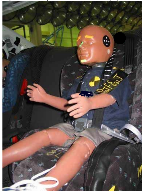
Figure 5. Frontal test for Booster A with seatbelt and harness with crotch strap
