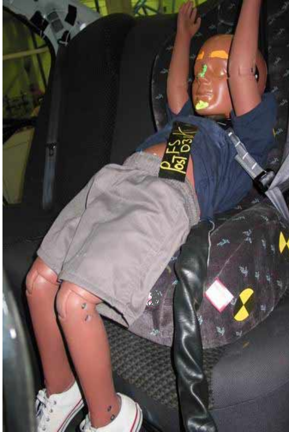
Figure 6. Frontal test for Booster A with seatbelt and harness with the crotch strap disengaged
