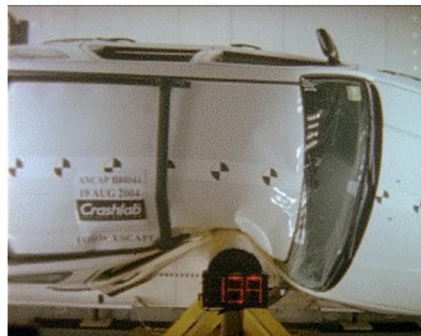
**Figure 3. Pole impact test at 29km/h (ANCAP)**
