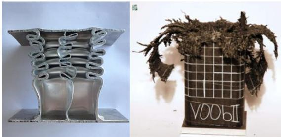
Figure 3: Comparison between plastic folding in metals (left) and fragmentation in composites (right) [5].
