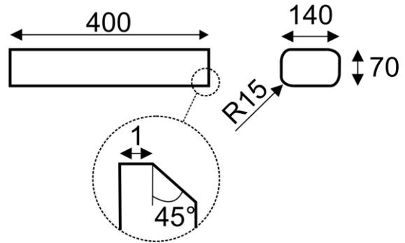
Figure 6: Specimen dimensions and Trigger configuration for an example specimen with a 1:2 Aspect ratio.
