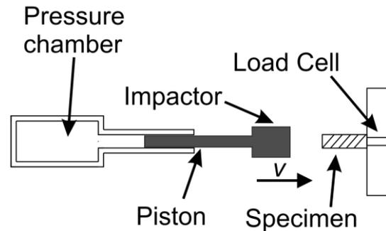
Figure 7: Impact test configurations.
