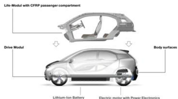
Figure 1: i3 vehicle architecture.
