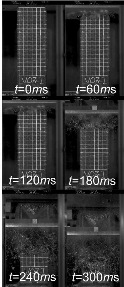
Figure 8: Deformation sequence for specimen V04 during high speed impact testing
