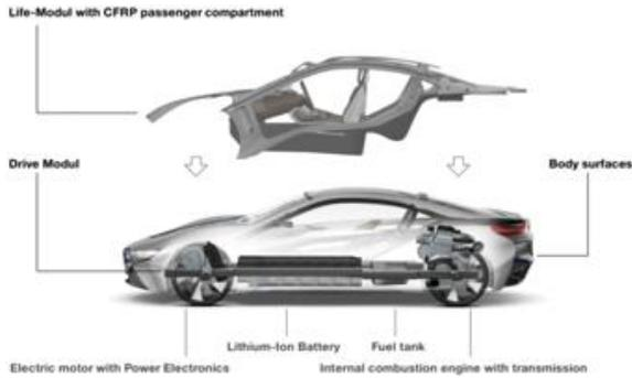
Figure 2: i8 vehicle architecture.
