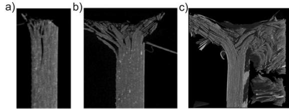
Figure 4a –c): Crushing fragmentation in a composite structure [7].
