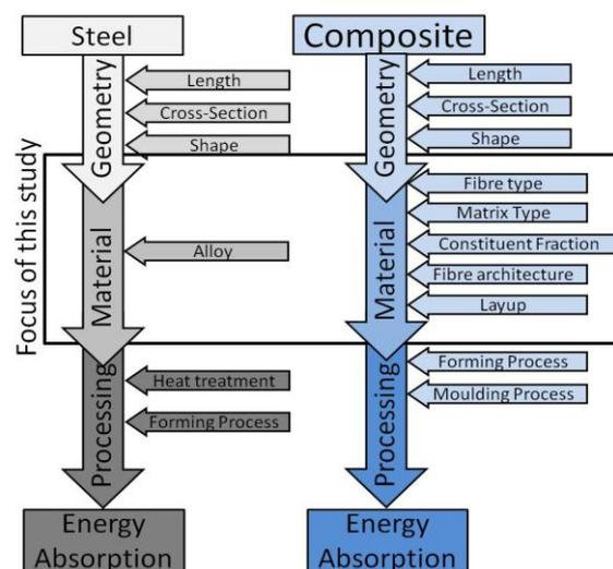
Figure 5: Comparison between typical design decisions affecting the specific energy absorption of a component.
