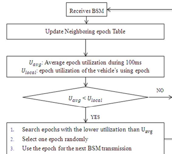
*Figure5.* Phase control algorithm
