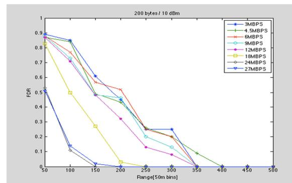
Figure3. Packet Delivery Rate vs Data rate
